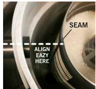
Figure 10. Align the Eazy seam to the centre of the overflow pipe.
