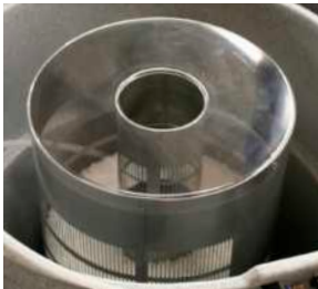
4) Eazy Mechanical Filter K1Micro is supplied in place in the Eazy section of your Nexus 320+.
